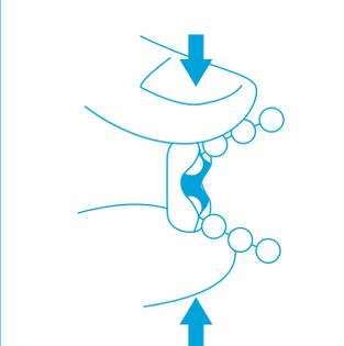
Hook the tip of the chain into the groove and pull it strongly to lock.
